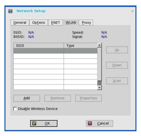
a Add—Use this option to add and configure a new SSID connection.
