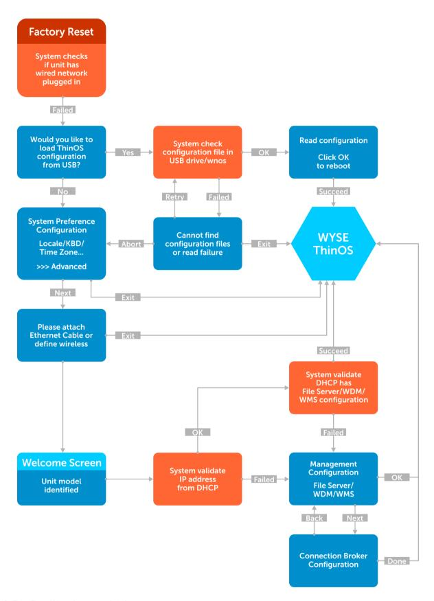
Figure 2. First Boot Wizard—network failure
