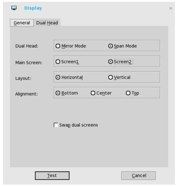
For Swap dual screens, when you set Main Screen to Screen2, an additional check box is displayed at the bottom of the tab that allows you to swap dual screens. If you clear the check box, the Screen1 is usually the left one or the top one in dual display. When you set Main Screen to Screen2, the main screen is changed to the right screen or bottom screen. If you select the **swap**
